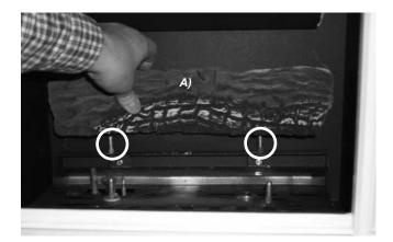
5) Place the 2 front logs on the front log locating pins. Ensure the back of both logs rest against the tabs.
